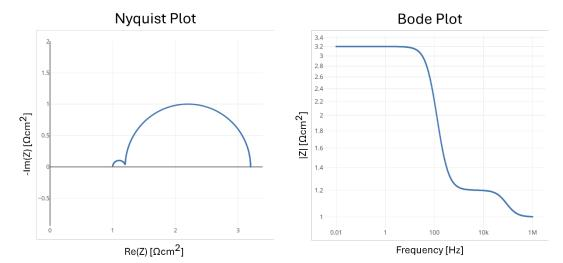
d) Changing the anode material results in changes in the anodic capacitance and resistance, therefore the new Nyquist and Bode plots are shown as:
