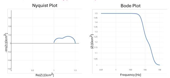
By comparing the Nyquist plots of the two different cells, it can be concluded that when the time constants of the 2 RC circuits are different enough (case 2), the 2 semi-circles are distinct, but when the time-constants are close (case 1), the semi-circles overlap.
